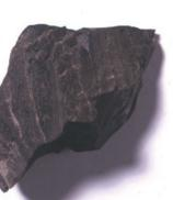
ploited using naturally-occurring fractures in the shale, which functions as the reservoir, source rock, and seal.
